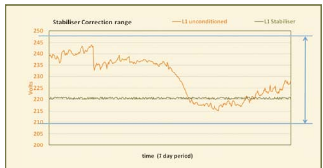
Figure 7: Response to variable supply: regulator correcting voltage to target output
